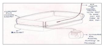
Figure 7: Open care converted as an incubator.
