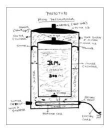
Figure 2: Prototype mini-pasteurizer.
